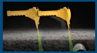
Holding the AML's handle parallel to the ground, scan the area of the undetectable buried object until one or both of the target indicators activate.
