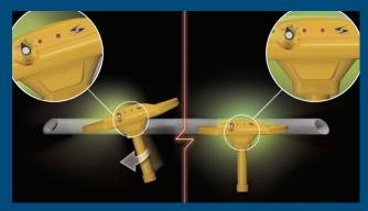
While the left or right target indicator is activated, rotate the AML until both LED target indicators light simultaneously, triggering the AML's tone and laser marker. This alert indicates that the pipe or object has been detected and that the AML is now parallel with the underground object.
