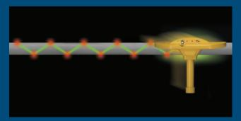
With the AML parallel with the pipe or underground object, you can now scan the entire length of the object's edge. As an alternative, utilize the "W" method of scanning by sweeping the area in a back-and-forth "W" motion, marking the object's location and run direction as it is tracked.
