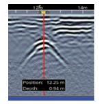
Use hyperbola-fitting to ensure accurate depth measurements and backup over the target to display its location and depth
